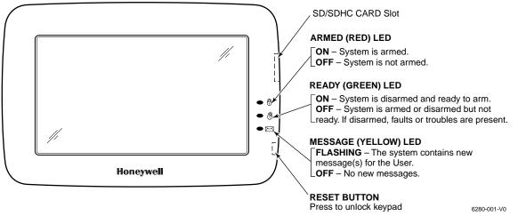
\*Note: If the EN50131 Display feature is enabled, the "Armed" and "Ready" status LEDs turn OFF after 30 seconds and the screen returns to the Home screen until a valid user code is entered.
